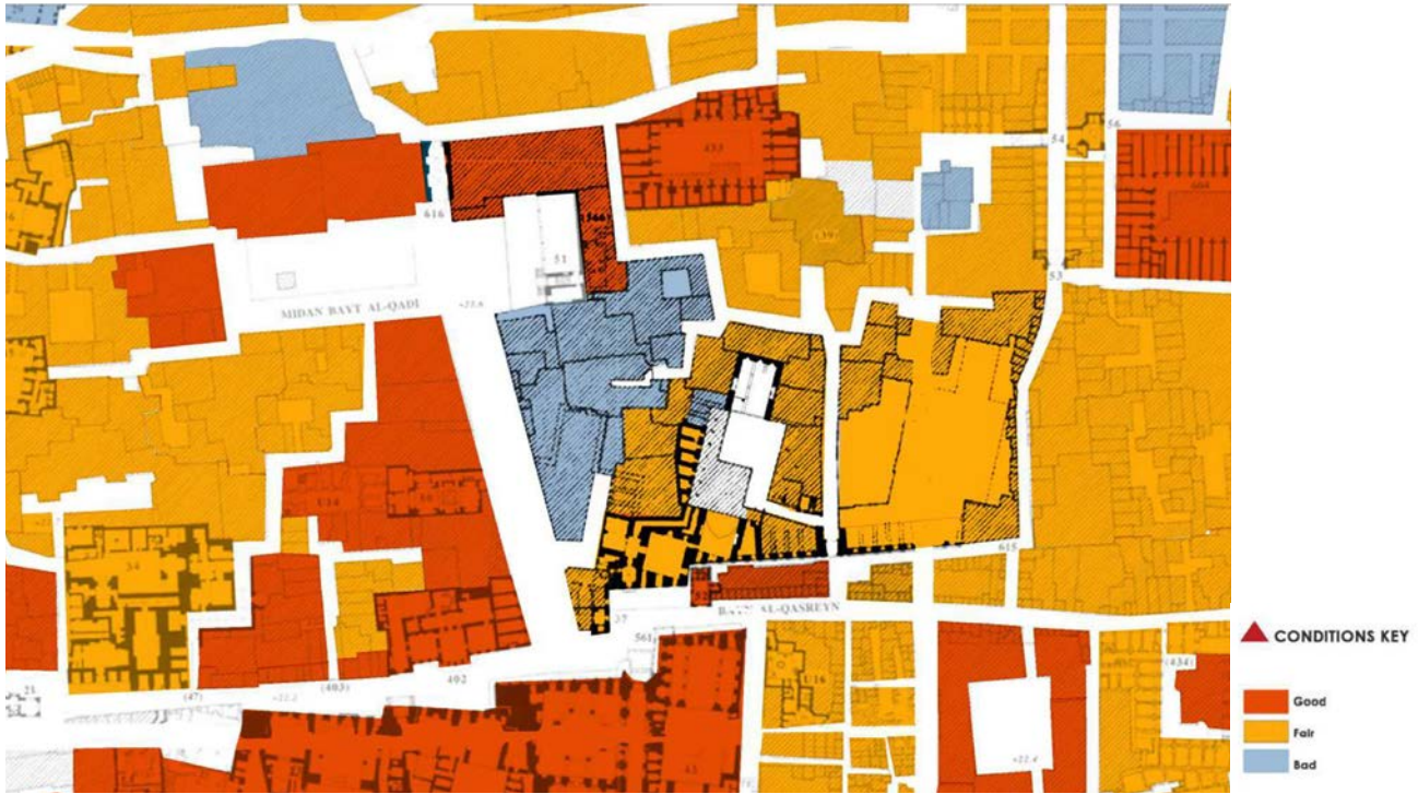
Conditions of the buildings in Al Gamaliya District. Source: Ministry of Antiquities, 2018. Edited by the Authors.
